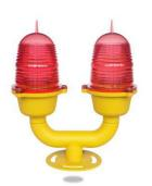
This Low-intensity Double light is a steady burning aviation obstruction light designed for marking top of obstacle that do not exceed 45 meters in height. Main-standby mode ensure the obstacle is always marked even one light fail.
